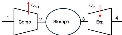
Figure 2.17: Simplified I-CAES block diagram
