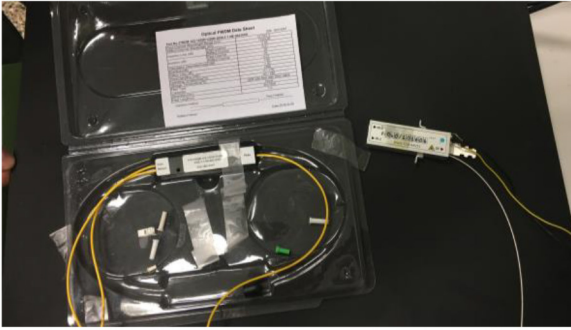
FIGURE 3. The AAVS1 Front-End device (on the right side of the picture) connected to the wavelength division multiplexer (on the left side of the picture) during the characterization performed before the test session.
