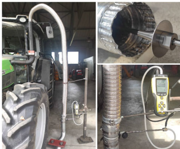
Fig. 2 Experimental arrangement of the tested tractor. Left: general view; top right: the gas probe; bottom right: the flow meter
