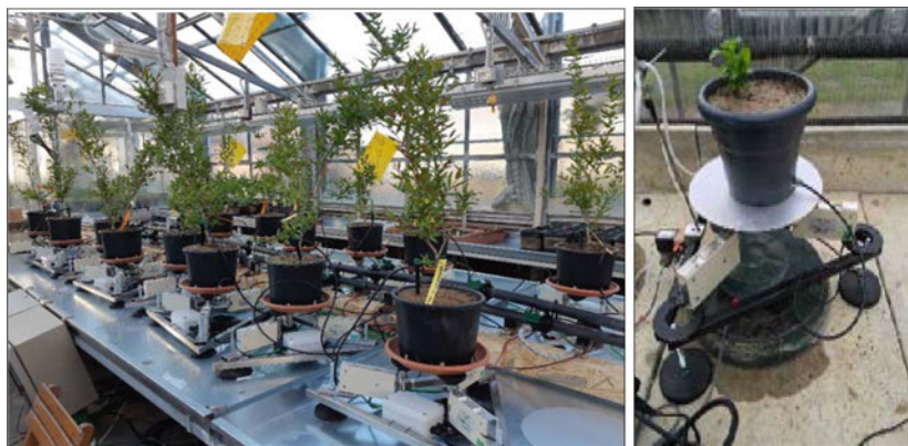
Fig. 1 The sixteen modules of the HTS platform integrated with the Time Domain Reflectometry (TDR) and the gravimetric (Lysimetry) segments, irrigated with the drip irrigation system
