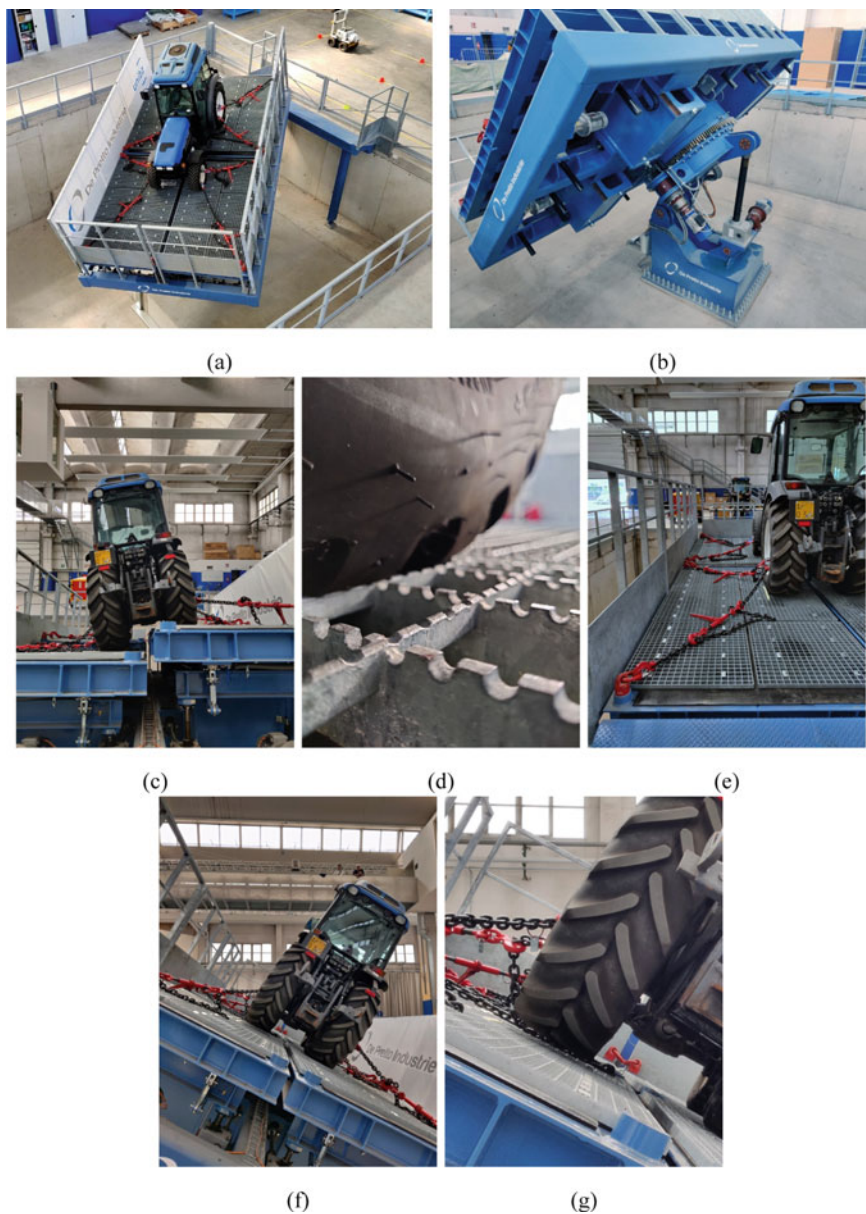
Fig. 2 Experimental test: (a) Stability test-rig and New Holland TN75V tractor, (b) test-rig rotational degrees of freedom, (c) plane conformation, (d) plate special metal grid, (e) tractor anchoring with chains, (f)(g) roll-over instability
