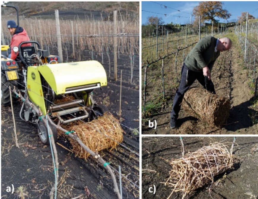
Fig. 2 a Vine shoots collecting and Roll Modular Fascine (RFM) production with the CAEB International QUICKPOWER 1230 round bale wrapping machine, b weight collecting of RFM, c low density RFM ( 100 \text{ kg/m}^3 )
