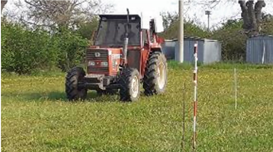
Fig. 6 Tractor during field tests. Antennas are visible on the tractor and passive RFIDs have been placed on obstacles all around the working area
