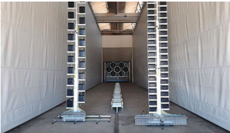
Fig. 5 View of the wind tunnel with the walls deployed from the entrance. The vertical patternators are on the foreground, and the horizontal one runs along the length. In the background, the fan array can be seen
