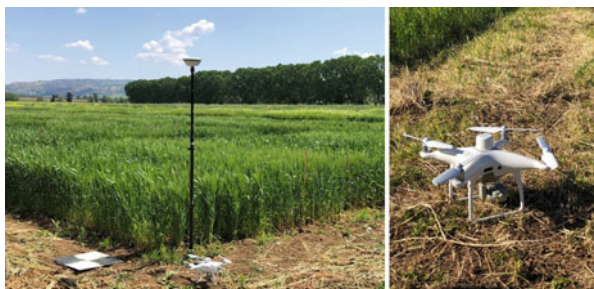
Fig. 2 Ground control point (GCP) and Leica GS12 RTK GNSS (left). The UAV DJI Phantom 4 Pro RTK (DJI Ltd., Shenzhen, China) (right)
