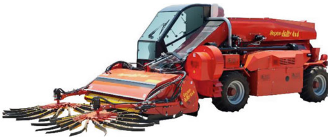
Fig. 2 GF Super Jolly 4 × 4 self-propelled mechanical harvester with driver's cab
