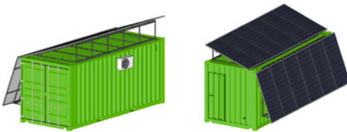
Fig. 1 Structure of a photovoltaic dryer for nutraceutical and aromatic plants
