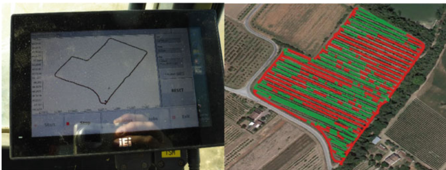
Fig. 2 The first part of the analysis at the Magliano experimental fields involved identifying the perimeter within which to do the surveys and identification of soil zones based on electrical conductivity
