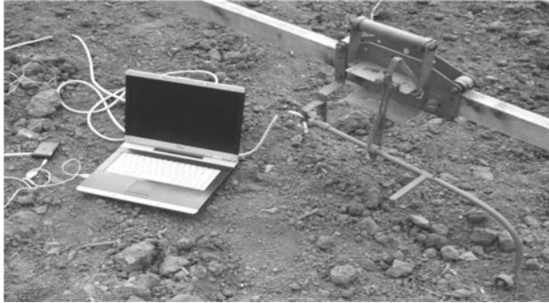
Fig. 3 Instrument for measuring longitudinal field profile
