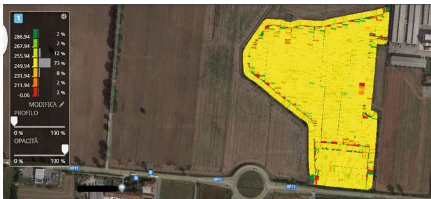
Fig. 2 Example of map of the dose (different colours represent the doses in L\ ha^{-1} ) distributed by the T2 operator (from the MyJohnDeere® management system)
