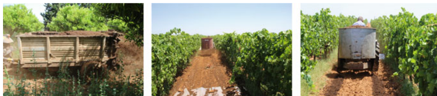
Fig. 1 Machines used to spread the solid fraction of digestate: the broadcast manure spreader used in the citrus orchard (left), the centrifugal broadcast spreader (center) and the localized spreader (right) used in the vineyard
