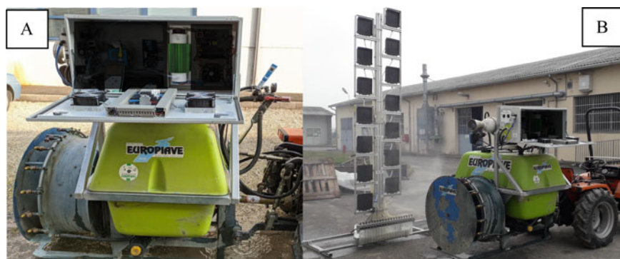
Fig. 1 (A) Mist-blower sprayer equipped with the ozone generator and linked to the tractor used for the trials. On the right of the ozone generator the Apera probe is visible; (B) OW sprayer during the test with the vertical test bench
