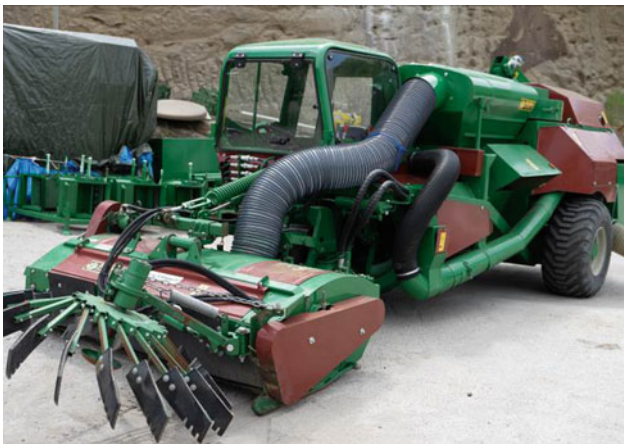
Fig. 1 FACMA Cimina 300S self-propelled vacuum harvester, with RM210 and driver's cab
