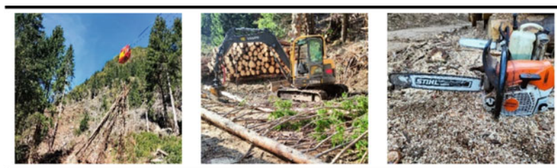
Fig. 1 Typology of used machines. Left: cable crane with mobile drive station; center: earthmoving machine equipped with hydraulic clamp; right: chainsaw
