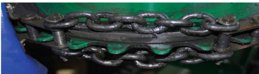
Fig. 3 Teeth of the wheel entered between the two sections of the ring chain
