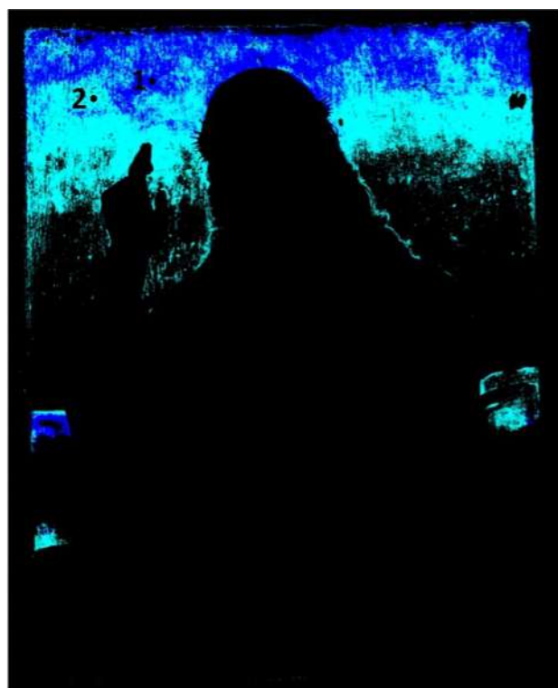
Figure 7. False-color map obtained from HSI VNIR data using the SAM algorithm, where light blue and dark blue pixels correspond to the distribution of Egyptian blue and ultramarine blue, respectively. Representative spectra of the two materials, on the right, were extracted from marked areas on the map.
