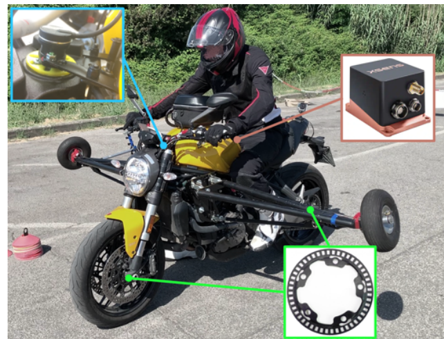
(a) The instrumented motorcycle with outriggers. The positions of the steering angle sensor, inertial measurement unit, and wheel speed sensors are shown.
