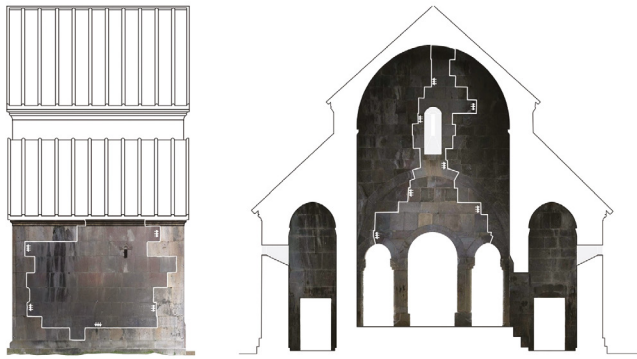
[fig. 17] Left: restoration visible in elevations 1 and 5 (counter-façade); right: the surface dressing of the phase 5: ygv2 (on the left) and ygv3 (on the right)
