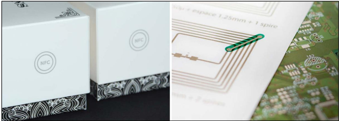
Figure 2. Micro-fibrillate cellulose food boxes with RFID tag printed on cardboard to communicate dietary properties to smart devices. Made by Stora Enso, 2016. Overall view and detail.
