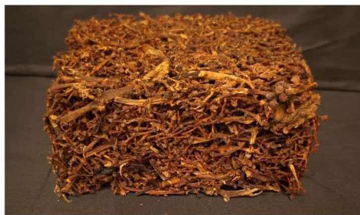
Figure 6. Image of the sample made entirely of grape stalks (T3_C3_L10). Its production was carried out using a WIKA pressure gauge reading of 760 \pm 10 \text{ kPa} and a 6 min microwave heat treatment (T3).
