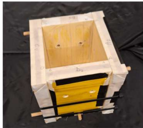
Figure 4. Image showing the parallelepiped wooden mold used during the experiments. The mold dimensions were 138 mm high, 173 mm wide, and 157 mm long, with a wall thickness of 26 mm. The mold was closed by a base and a cap, both with the same wall thickness, measuring 121 mm wide and 105 mm long.
