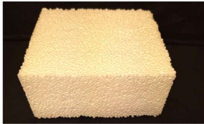
Figure 3. Image of the sample made entirely of expanded PLA (E-PLA). It was produced at a WIKA pressure gauge reading of 450 \pm 10 kPa and subjected to a 6 min microwave heat treatment.
