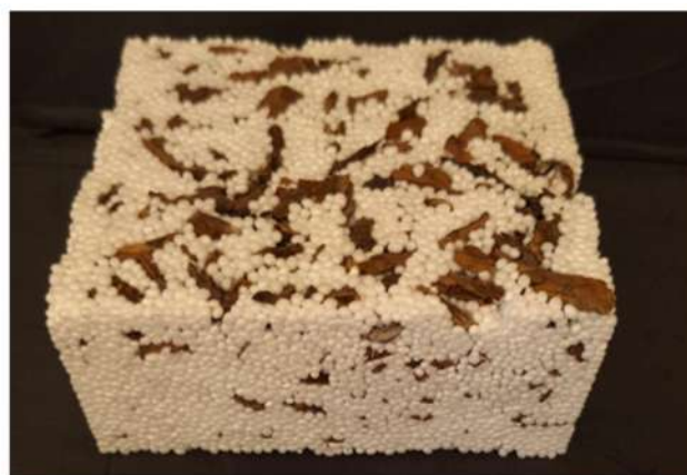
Figure 5. Image of the sample made from 40% spruce bark (T3_C1_L4). Its production was carried out using a WIKA pressure gauge reading of 760 \pm 10 kPa and a 6 min microwave heat treatment (T3).
