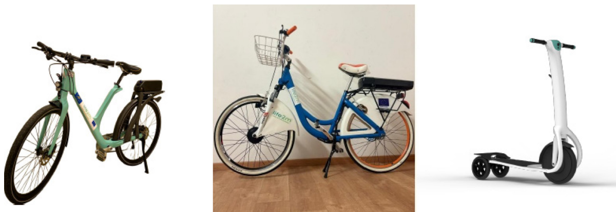
Figure 1. Microvehicles implemented for the LIFE2M project: prototypes of e-bikes (left), retrofitted muscular bikes (centre) and Leonardo e-scooters (right), which integrate HSC-based accumulators
