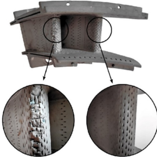
Figure 2.3: Portion including two nozzle guide vanes (NGVs) from a high-pressure turbine in a turbofan engine [38].
