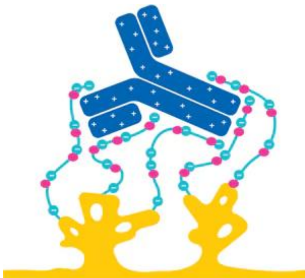
Fig.39: Stationary phase of Eshmuno® CMX Chromatography resin.
