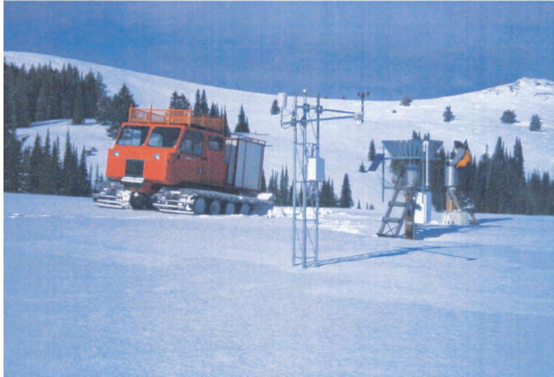
Figure 6.15: Climate, snow, and precipitation measurement site near fir forest in the southern, higher-elevation region of the Reynolds Creek Experimental Watershed, from Slaughter et al. (2001).
