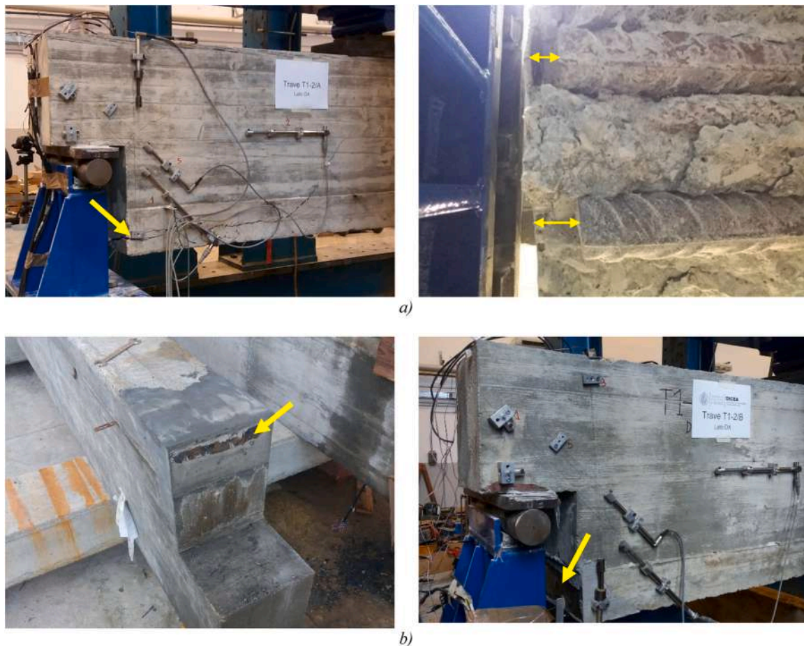
Fig. 15. a) Failure mode of specimen T1–2A* with diagonal crack and identification of the slippage of the bottom longitudinal bars (yellow arrows). b) View of specimen T1–2B in an upside-down position before launching (left) and on the testing machine (right): the arrow identifies the anchorage plate.
