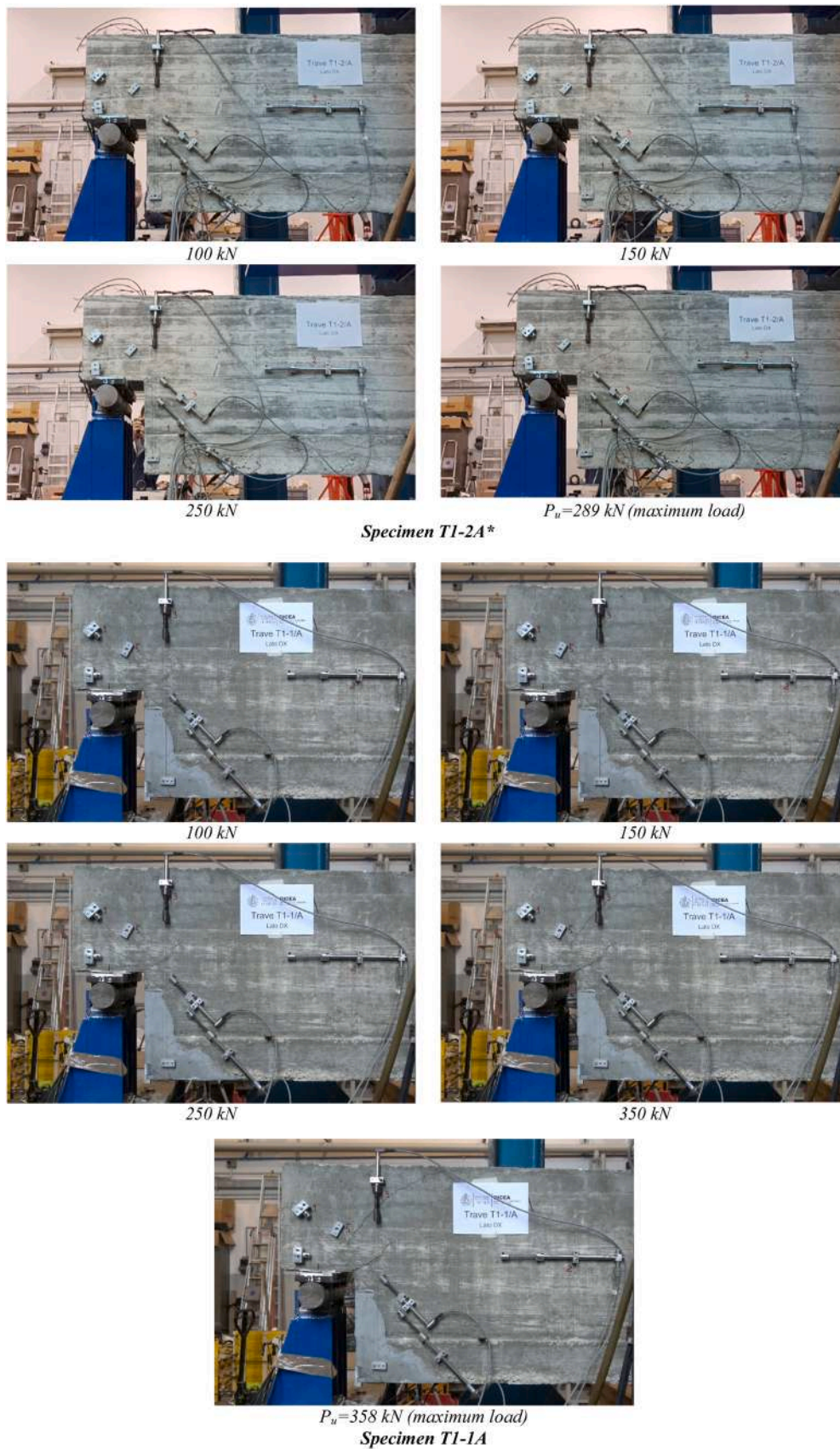
Fig. 17. Crack pattern at different levels of the applied external load.
