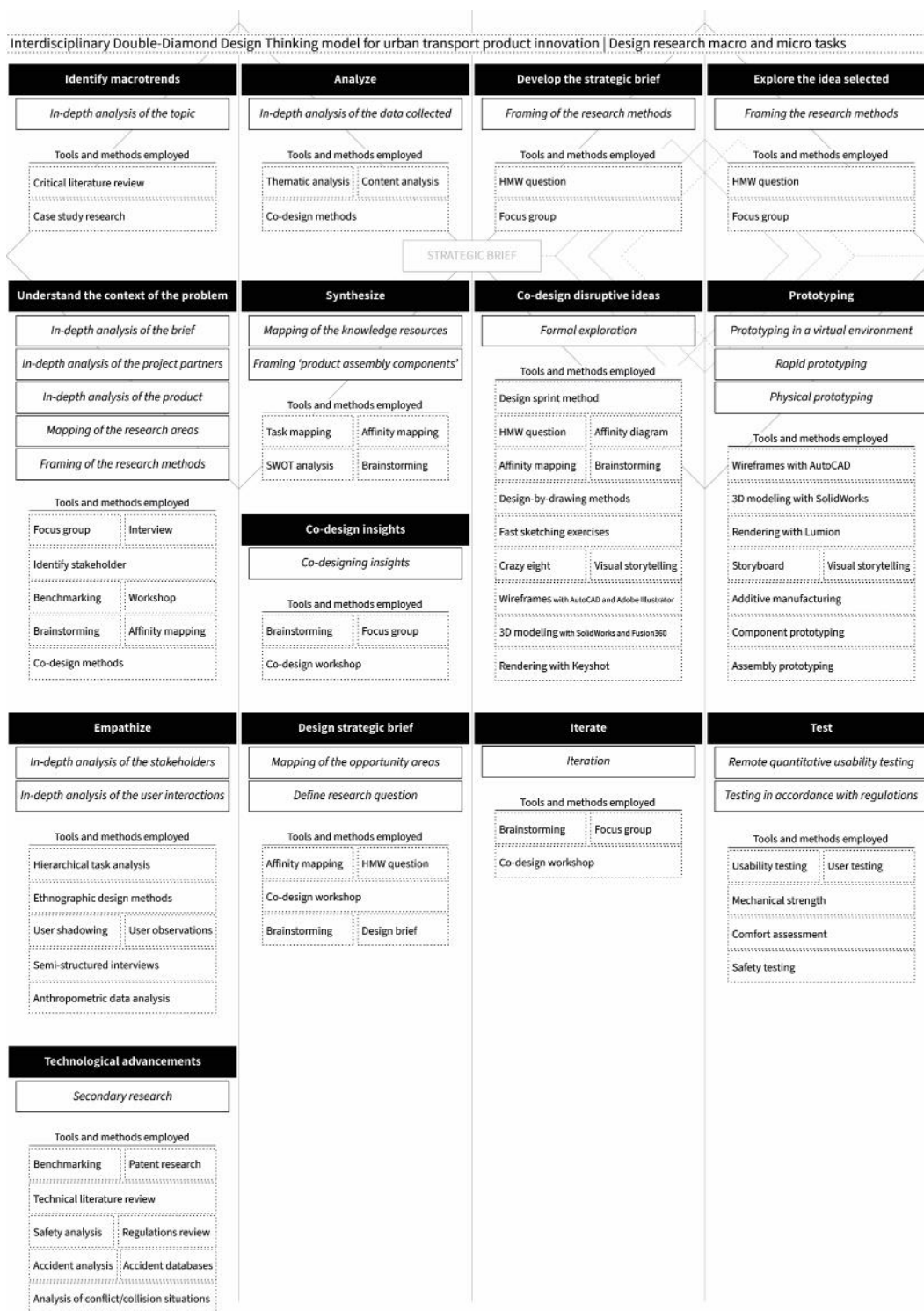
Figure 16. Interdisciplinary Double-Diamond Design Thinking model for urban transport product innovation. The figure presents the design research macro- and micro-tasks and tools and methods to employ for mobility product innovation. Re-elaboration of the “Double-diamond design thinking model” [29].
