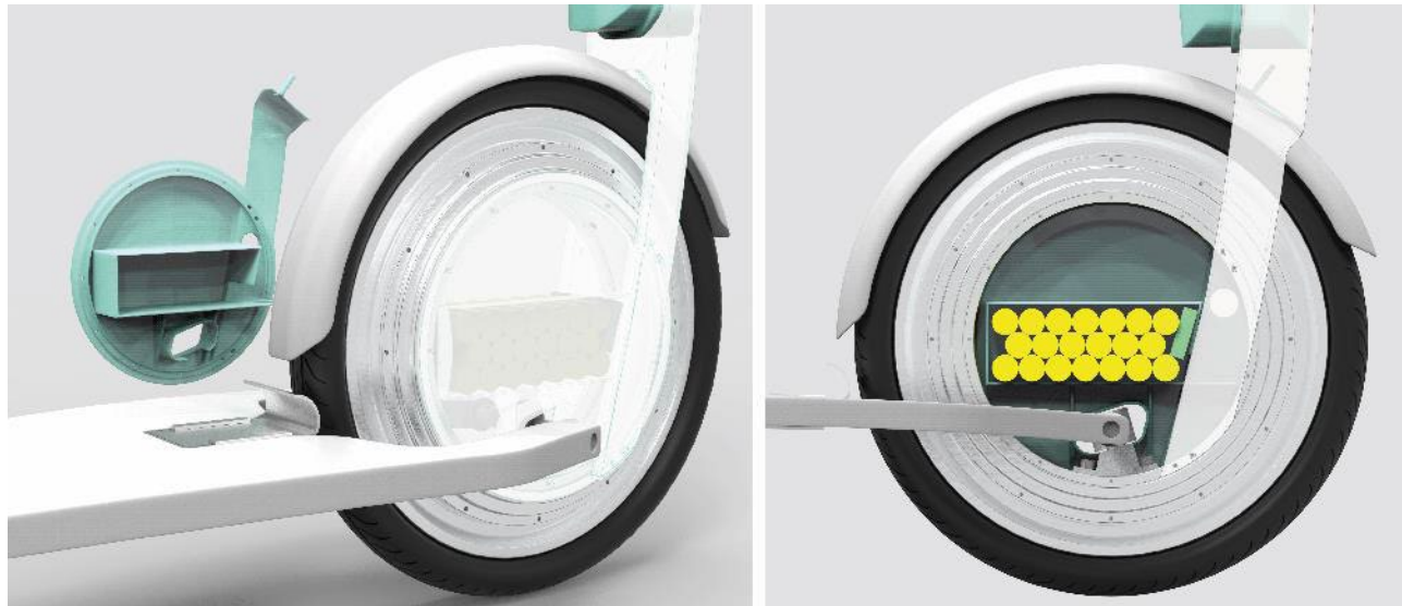
Figure 11. Overview of the fixed battery case configuration.
