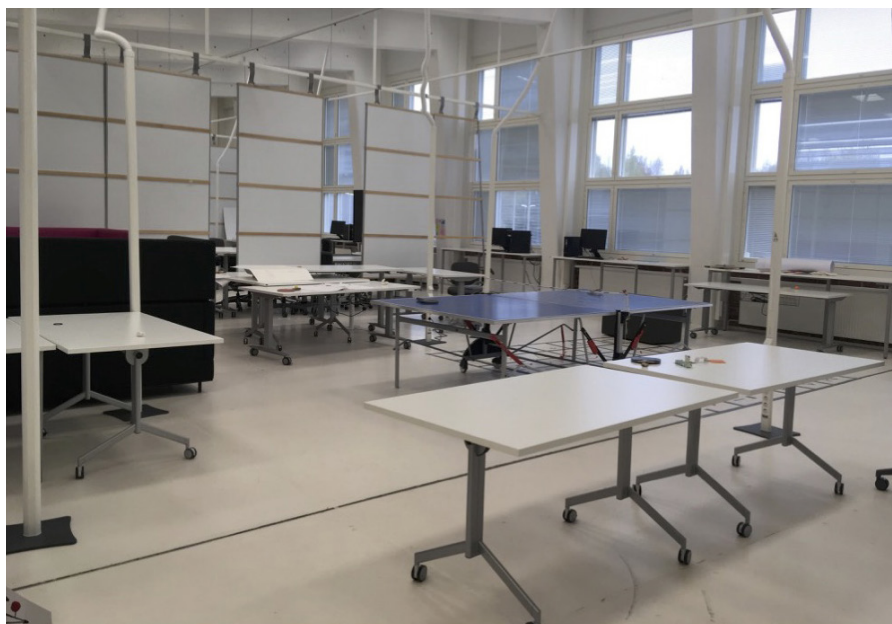
Fig. 25.3 - The space has room dividers, but acoustically they are inadequate (Sulkamo T.)
