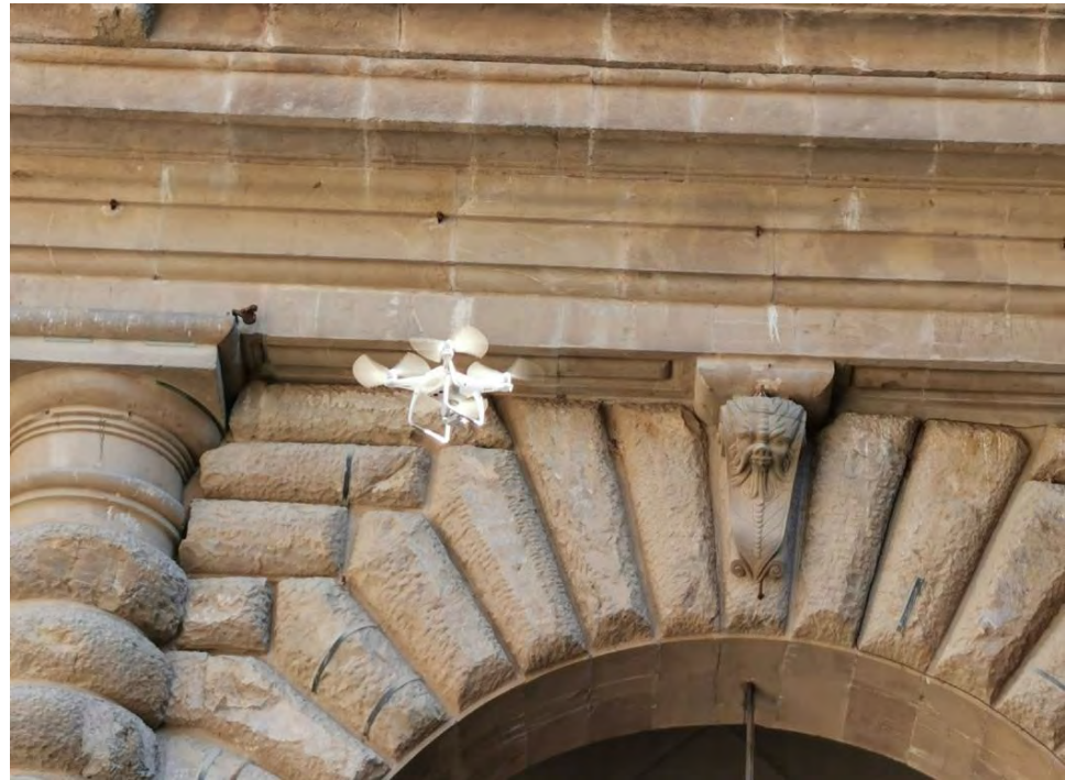
Figure 6. A photo of the DJI Phantom Pro UAV in flight, surveying the “Cortile dell’Ammannati”.
