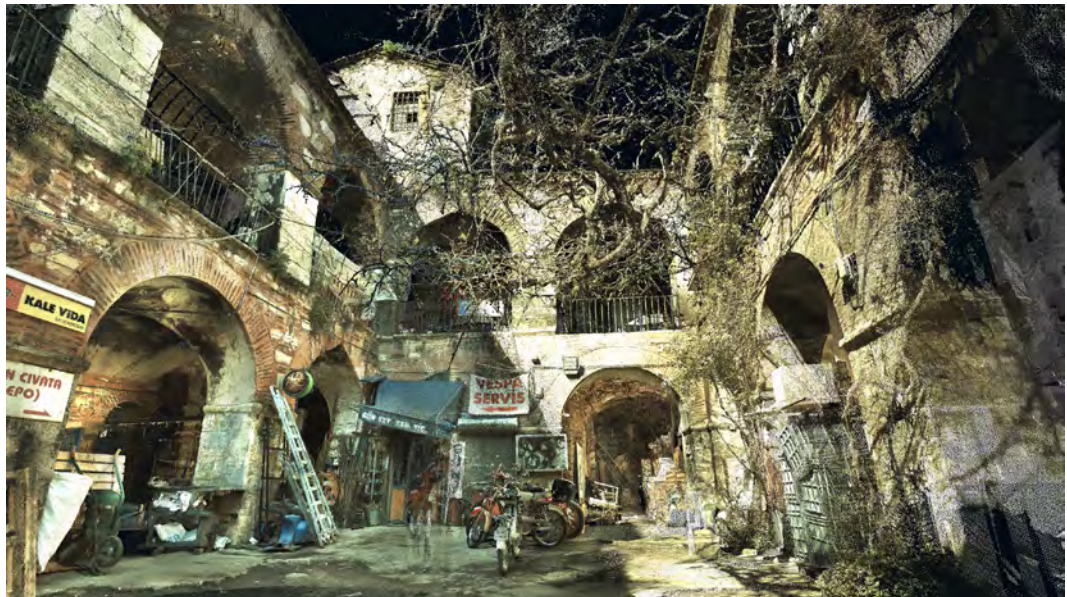
Fig. 7. Perspective view in the Caravansary of the aligned point cloud.
