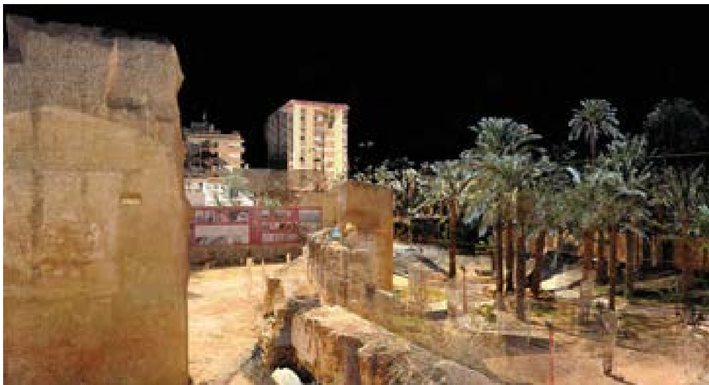
↑ Fig.06 Digital database Colorimetric view of the point cloud of the complex.
