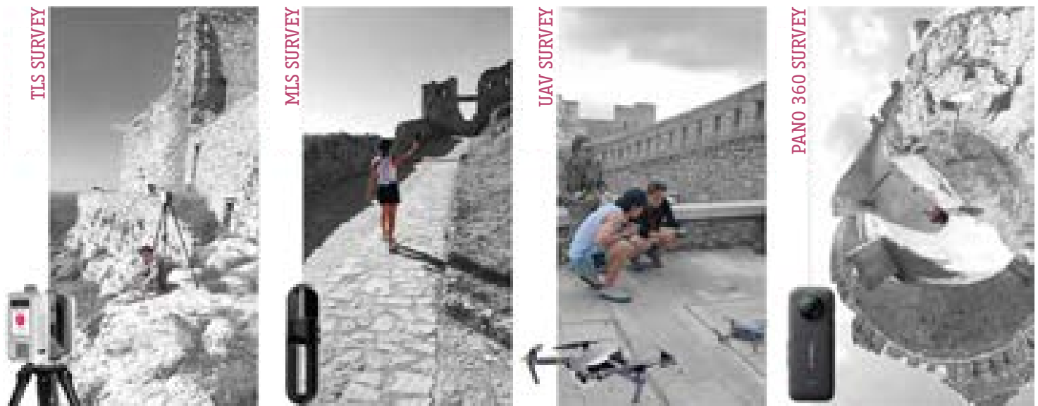
↑ Fig. 05 Survey techniques Integrated survey techniques for the documentation of Morella Castle using terrestrial laser scanning (TLS), mobile mapping (MLS), drone-based (UAV), and 360° panoramic imaging.
