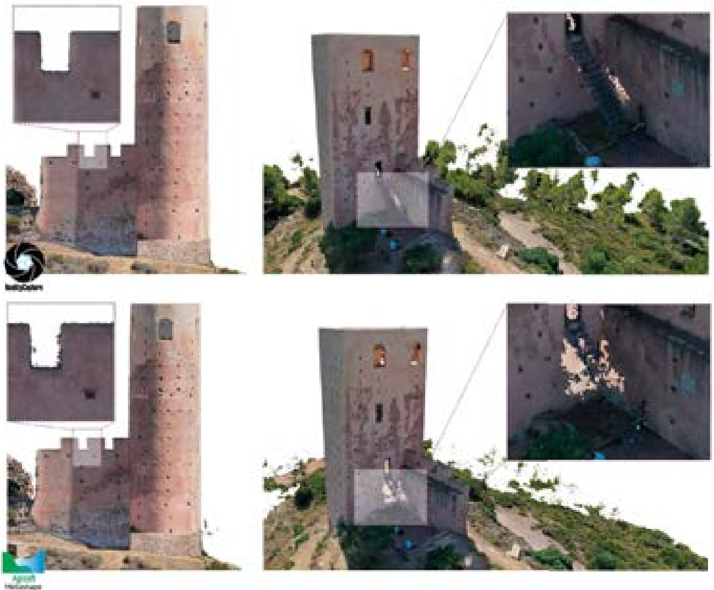
Fig. 07 Comparison of Photogrammetric Outputs Visual comparison of 3D models generated with RealityCapture (top) and Agisoft Metashape (bottom). The images highlight differences in texture resolution, mesh completeness, and the handling of problematic areas such as shaded zones and surfaces with low texture detail.
