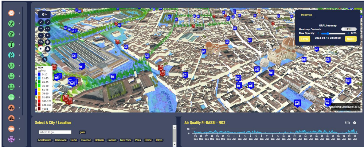
Figure 5. 3D multi-data map widget used to represent the smart city digital twin of Florence, Italy.
