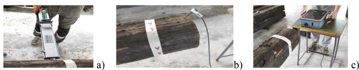
Figure 3. Application of NDTs: a) the drilling resistance (DRM); b) acoustic; c) vibrational methods.
