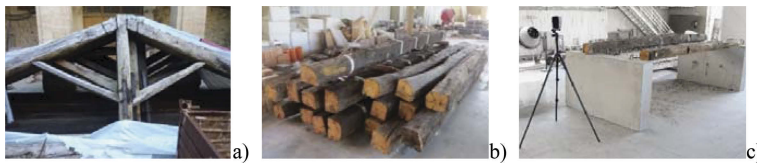
Figure 1. a) Timber trusses extracted from the lyceum gymnasium Bernardino Telesio, Cosenza (Italy); b) Timber rafters stored in the DINCI Laboratory, Rende (CS); c) Survey of two rafters with laser scanner.
