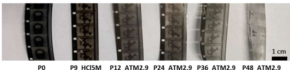
Fig. 25 Real motion picture films before the degradation protocol (P0), after a 9 days-long exposition to HCl 5M atmosphere (P9_HCl5M) and after ATM2.9 protocol (P12, P24, P36, P49_ATM2.9).
