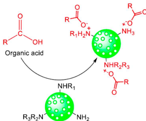
Fig. 2 Acid/base reaction scheme between PEI and acetic acid [9].
