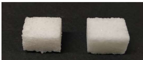
Figure SI_6. Photograph of the obtained PDMS_SC sponge (left) compared with the pure sugar cube (right).
