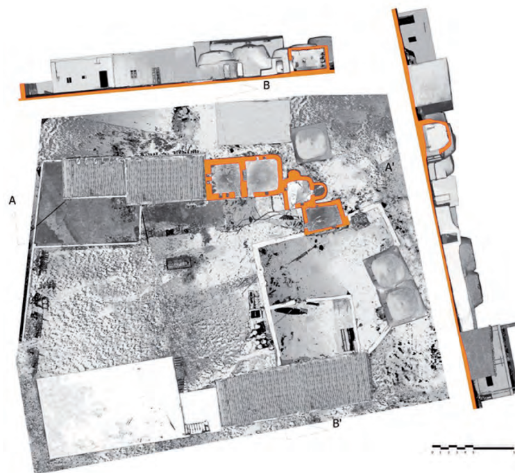
Fig. 3 Considering the laser scanning survey of a single dwelling, it is instead possible to distinguish larger and smaller modules (the first are generally used for dwellings or as stores, the second as kitchens, ovens or secondary rooms), to identify the open areas associated with the modules, ascertain the position of the mastaba and indicate the presence of external dividing walls (plan and elevation of the dwelling studied in Joub Maadi village, graphics elaborated on the basis of a laser scanning survey) (© Geomatics for Environment and Conservation of Cultural Heritage Laboratory)
