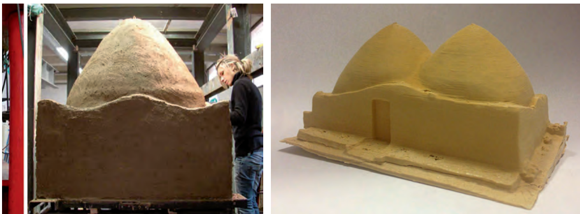
Fig. 6 Different 3D solid models were realised for different purposes: on the left, an earthen scale model building used for analytical and numeric assessment of the static performance of the devices based on specific hypotheses (Paglini et al. 2009b); on the right a small-scale 3D model printed using a coloured filament, made for communication purposes (didactic, exhibitions, support for disabled people, etc.) (© Geomatics for Environment and Conservation of Cultural Heritage Laboratory)
