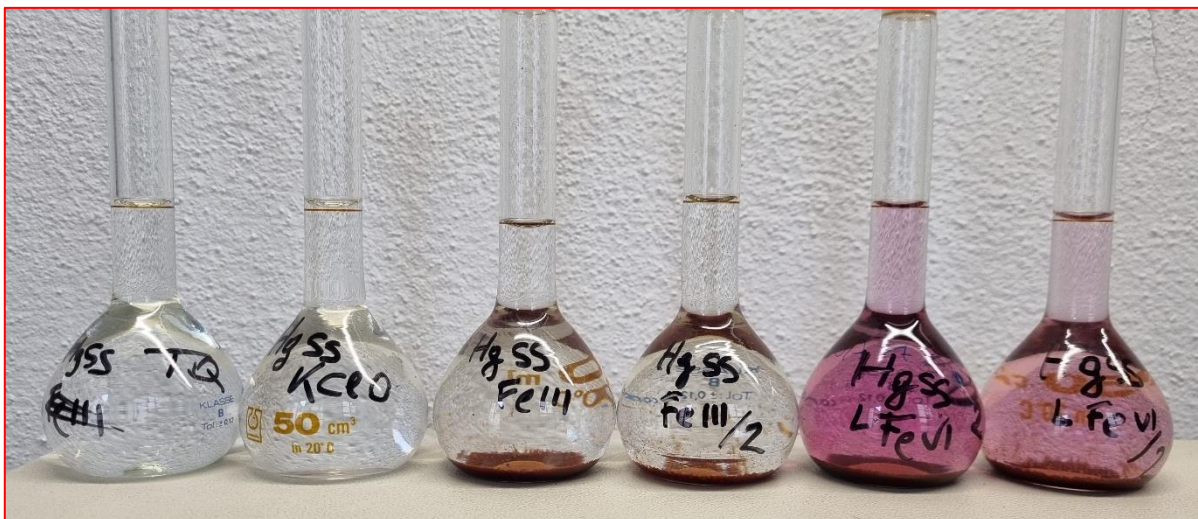
Figure 2.4: photo of some HgSS samples in 50 cc flasks after the addition of different reagents. The typical violet color resulting from the ferrate addition is clearly visible on the right flasks.
