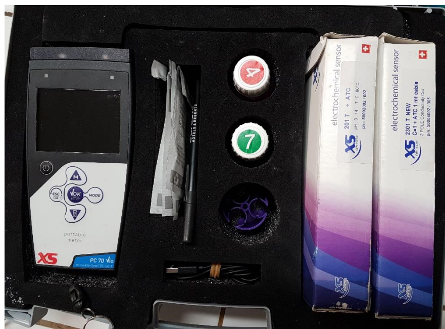
Figure 2.6: photo of the PC 70 Vio multimeter used for pH, electrical conductivity and T^\circ of the treated samples.
