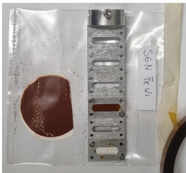
Figure 2.15: photo of one of the 47 mm filter cut, with the cut portion enclosed in Kapton tape and mounted over one of the free slots available in the aluminum sample holders.
