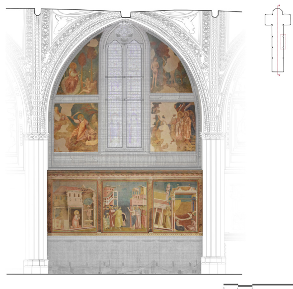
Fig. 2. Example of the digital survey of the Upper Basilica of Assisi, obtained through laser scanning and integrated with photogrammetric data, focusing on one of the bays (graphic elaboration by Roberta Ferretti).
