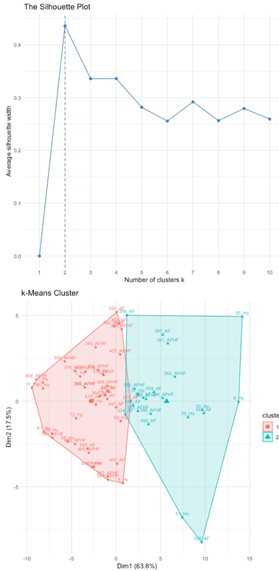
Figure 4.10: Above: Silhouette analysis to detect the best number of clusters to be used in cluster analysis. Below: results from the k-means clustering algorithm.
