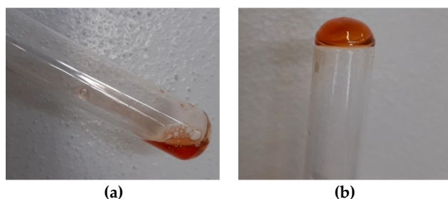
Fig. 3. Sol-gel transition. Sol form at 25 °C (a) and gel form at 37 °C (b).
