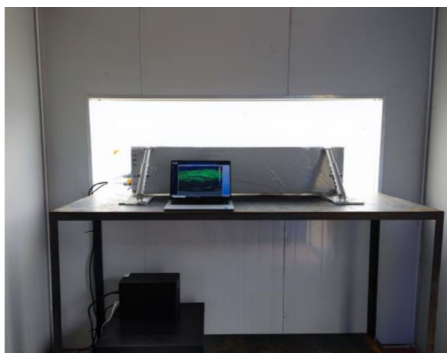
FIGURE 7 GB-InSAR system employed in the emergency monitoring.
