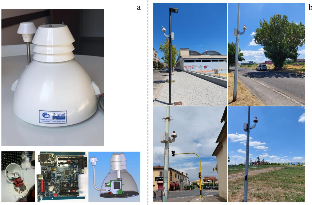
Figure A2. Pictures of the AirQino low-cost air quality monitoring station: (a) layout of the unit and internal motherboard; (b) unit's installation within Prato municipality.
