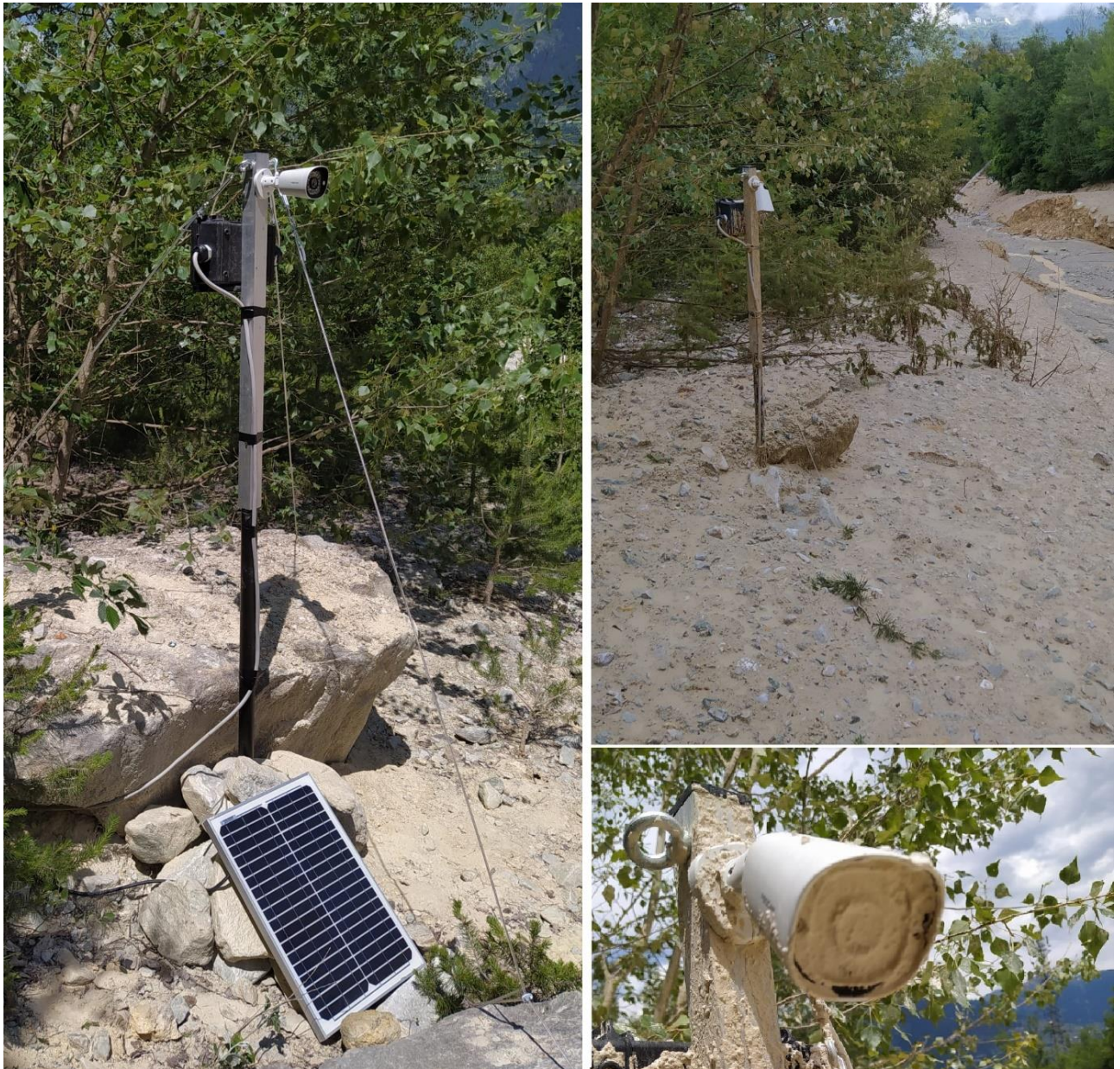
Figure 3. 12: a camera for debris-flow video recording before (left) and after (right) being hit by a debris-flow event in the 2021 debris-flow season at Illgraben (source: Giacomo Belli).
