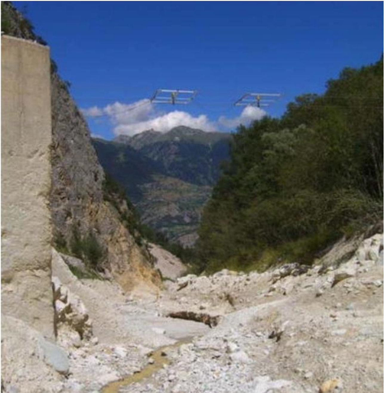
Figure 3. 9: two radar altimeters suspended over the channel at CD 10 for debris-flow detection (source: Badoux et al. [2009]).
