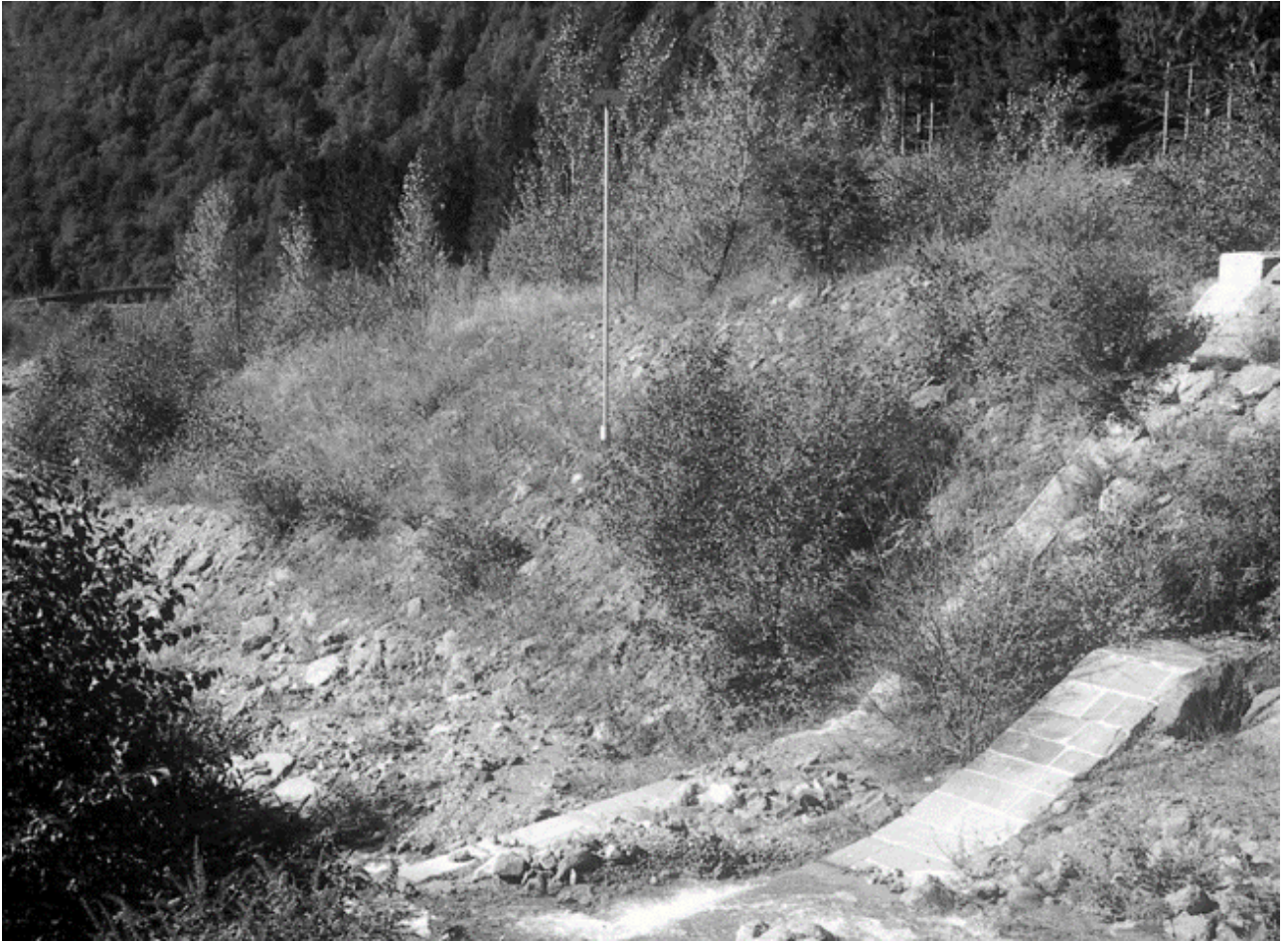
Figure 1. 20: ultrasonic sensor for flow depth measurement suspended over the channel at a check dam (source: Arattano and Marchi [2008]).
