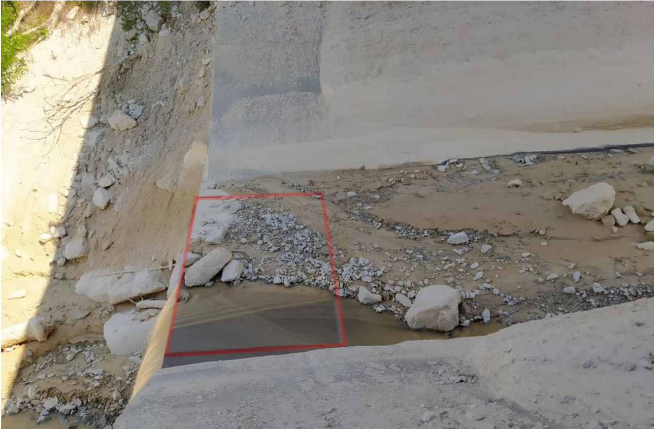
Figure 3. 10: photo of the 4×2 m force plate (highlighted by the red rectangle) deployed at the brink of CD 29 at Illgraben (source: Giacomo Belli).
