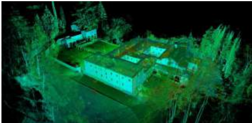
Fig. 4 The cloud of points of the laser scanner survey of the San Vivaldo convent.
