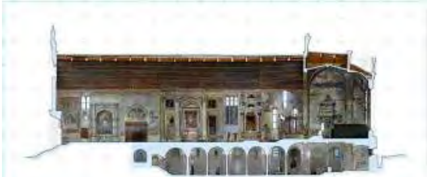
Fig. 5 Verona, Basilica of Saint Fermo. Longitudinal section (north side) and orthophoto of the northern side (Survey: Geogrà, 2016- 2018. Courtesy of: Parish of Saint Fermo, Diocese of Verona).
