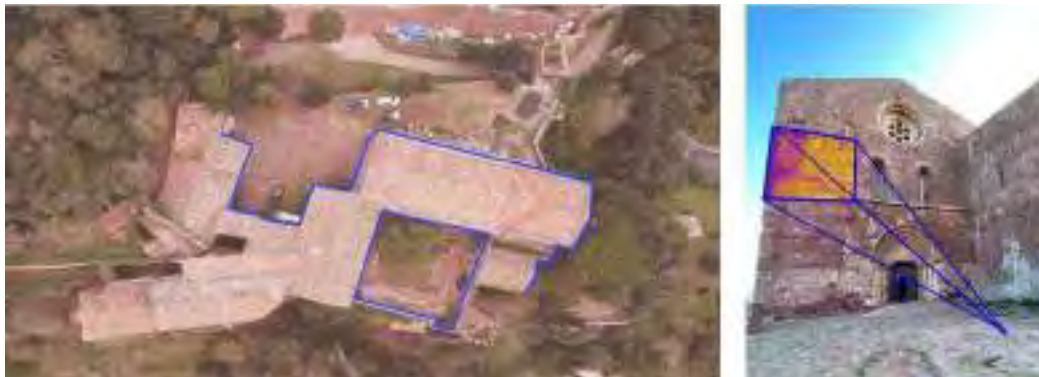
Fig. 2 Left) Aerial image of the monastic complex of Sant Miquel d'Escornalbou with the IRT investigated areas highlighted in blue. Right) thermographic long-range shot using thermal camera (credit: Sofia Brizzi).
