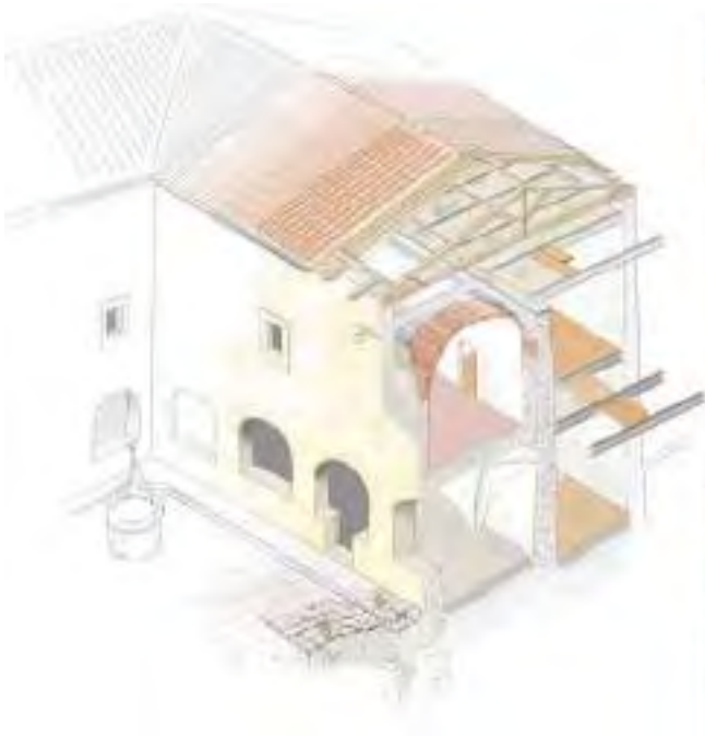
Fig. 8 Graphical Interpretative models, constructive sections (elaboration by Luca Vespasiano).
