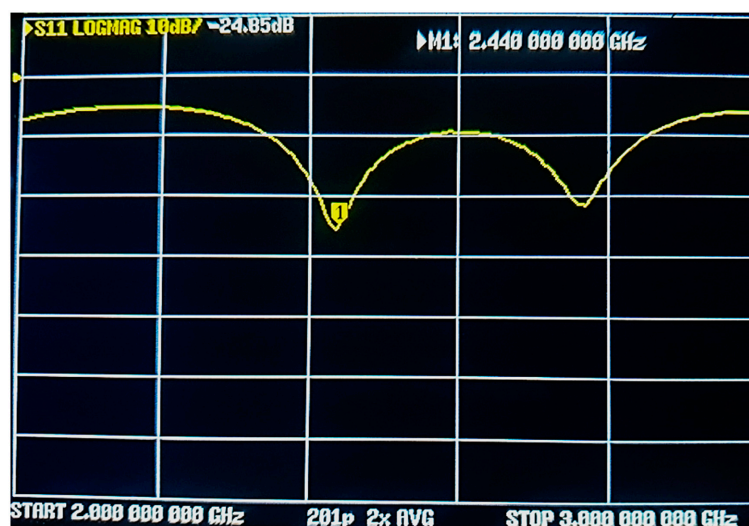
Figure 10. Input matching (S11 return loss) of the coaxial air-cooled applicator prototype measured with a vector network analyzer. The yellow curve represents the magnitude of the reflection coefficient S11 (in dB) as a function of frequency, from 2.000 GHz (START) to 3.000 GHz (STOP), with a vertical scale of 10 dB/division. The triangular marker (►M1) indicates the minimum return loss of -24.85 \text{ dB} at 2.440 GHz, confirming excellent impedance matching at the operating frequency.
