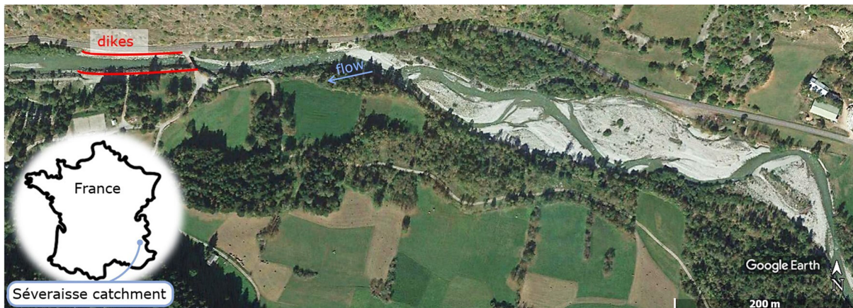
Figure 1. The Séveraise River, south of France; 44^{\circ}49'28'' N, 6^{\circ}9'6'' E. The reach framed in the photo has a slope of about 1.5% and a daily discharge of 10\text{--}30\text{ m}^3/\text{s} . The upstream part of the reach has a braided morphology, channels adjustments occur in the plain, planimetric sorting is present (poorly sorted sediments D_{50} = 37\text{ mm} , D_{84} = 113\text{ mm} ; patches of fines and coarse deposits). Downstream embankments force the river to a narrow single-thread morphology characterized by vertical channel adjustments, armoring ( D_{50} = 110\text{ mm} , D_{84} = 303\text{ mm} ), and no planimetric changes nor sorting.
