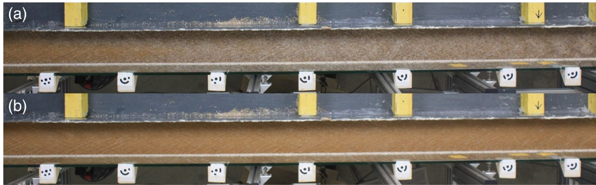
Figure 5. Extended sorting patterns characterizing some bed stages of Run 3; the central 2.8 m of the flume length are framed, the flow is from left to right. (a) A coarse-grained bed state, instant: 15 hr, 29 min. (b) A fine-grained bed state, instant: 15 h, 37 min.
