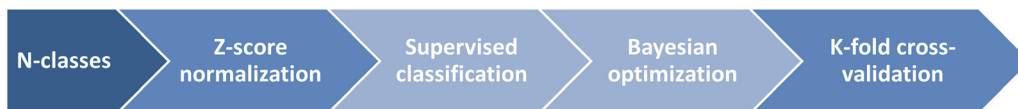
FIG. 1. (Color online) Workflow of machine learning experiments. The five-steps procedure applied for each artificial intelligence experiment is depicted. After z-score normalization, three supervised classifiers were trained and hyperparameters tuning was performed with Bayesian optimization. Models were validated with K-fold cross-validation (K = 10).
