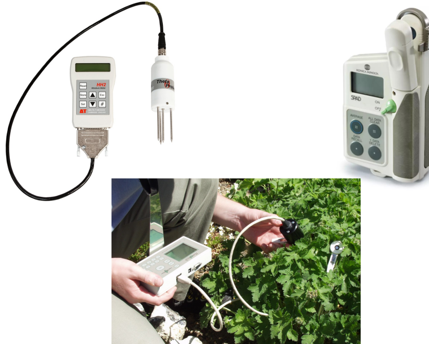
Figure S24: Instruments used for substrate and plant measurements during the experiment: HH2 Moisture Meter (Delta-T Devices, Cambridge, UK) for substrate volumetric water content (VWC) and pore water electrical conductivity (ECp); SPAD-502Plus meter (Konica Minolta, Osaka, Japan) for leaf chlorophyll content; and Handy PEA+ fluorimeter (Hansatech Instruments, Norfolk, UK) for chlorophyll fluorescence (Fv/Fm).
