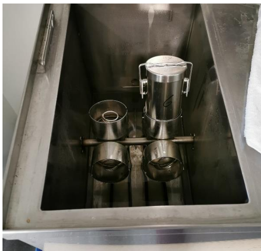
Figure IV.6: Laundrometer containing eight slots for individual washing pots with a capacity of 500 mL. Once placed in the instrument, the washing containers revolve around a horizontal axis.
