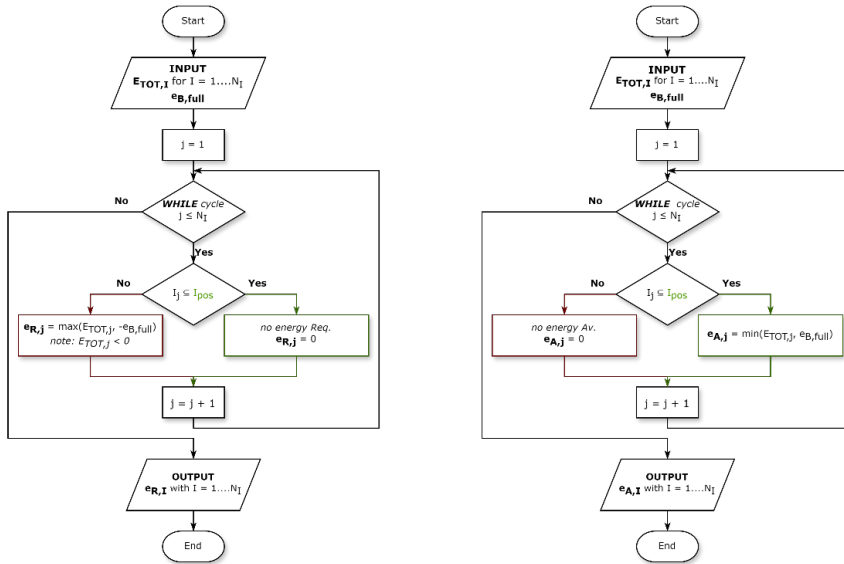
Figure 5.8: Flowchart of the first step of the rule-based algorithm. The left and right branches illustrate, respectively, the procedure to determine \bar{e}_R and \bar{e}_A .
