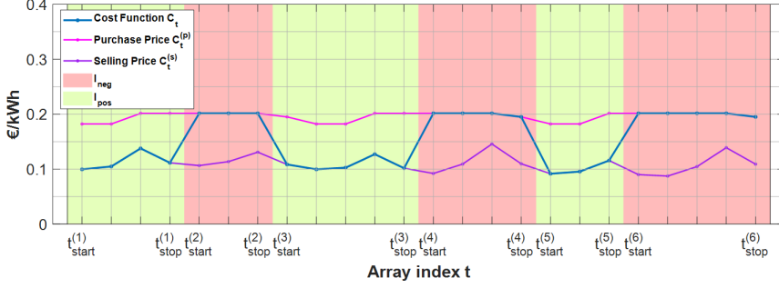
Figure 5.6: Example of derivation of the energy price array \bar{C} , given the energy profile in Figure 5.3
