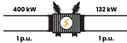
Figure 7.6: Representation of a transformer in p.u.
