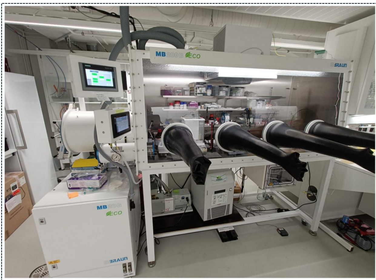
Figure 3.3. The glovebox used for the fabrication of PSCs at the University of Tampere, Finland.
