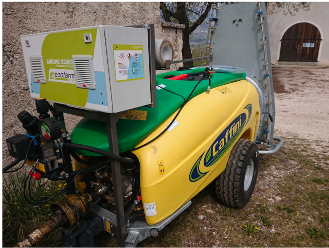
Fig. 1. Trailed-coupled sprayer of the firm Caffini (Patù, Verona – Italy) equipped with an ozonator of the firm Ecofarm Storti (Verona – Italy).
