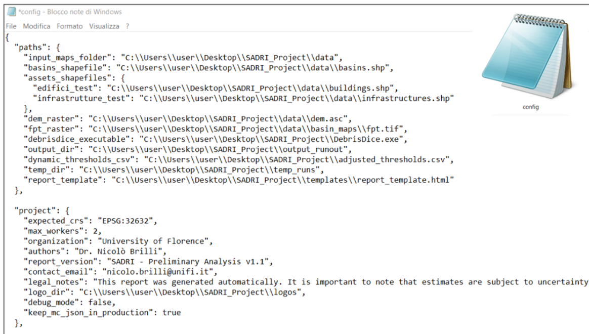
Figure 4. Example of config.json file structure for two types of sections (paths and project) for SADRI framework
