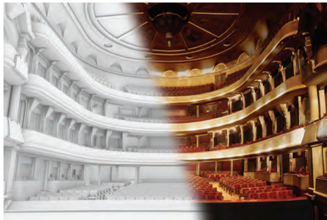
Fig. 2 - Concept of Aura project. The main hall of the Lviv Opera House depicting the interaction between the two 3D models: on the left the one intended for auralization and on the right the one for visual rendering.
