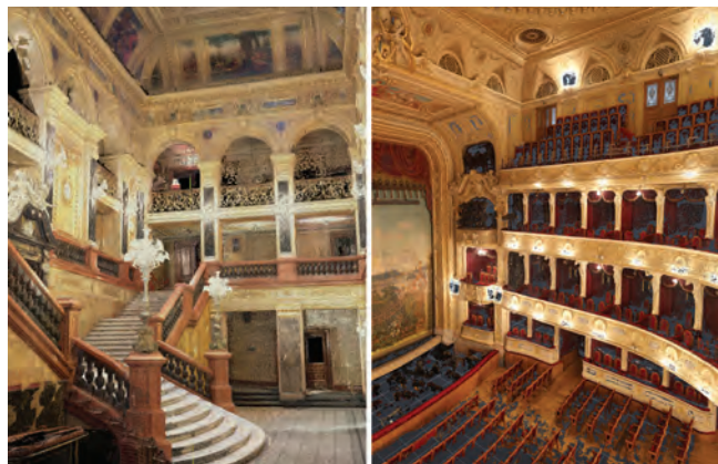
Fig. 07 – Colored point cloud of the foyer and main hall of the Lviv Opera House, developed from laser-scanner and photogrammetric surveys, respectively.
