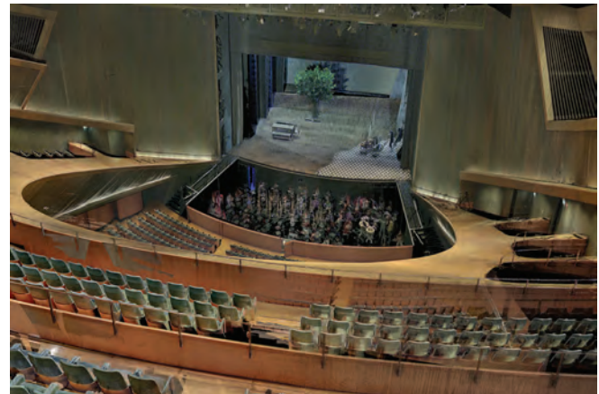
Fig. 05 – Colored point cloud of the main hall of the Berlin Konzerthaus developed from laser-scanner surveys.
