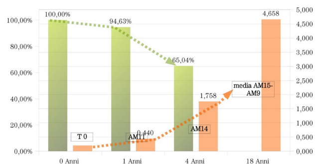
Figure 12: White marble, summary of the results: water absorption values and reduction of the effectiveness of the water repellents
