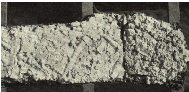
Fig. 14. Ravenna, St. Apollinare the New, preparatory cocciopesto layer of the mosaic of Agnellus (on the right) and preparatory layer made of a mortar rich in lime of the mosaic of Theodoric (on the left) (Bovini 1971). Foto SABAAR.
