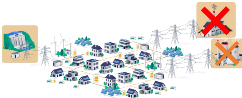
Figure 1.4: Distributed energy system
