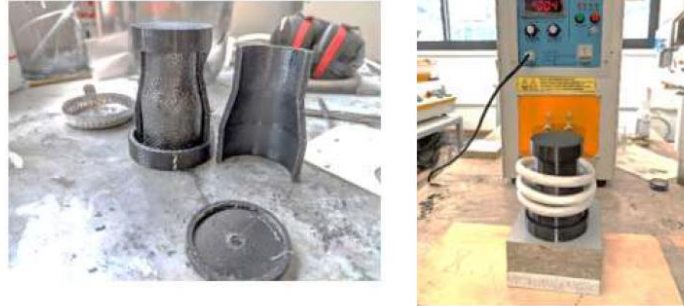
Figure 7. An example of a mandrel obtained using a novel wax-based blend.
