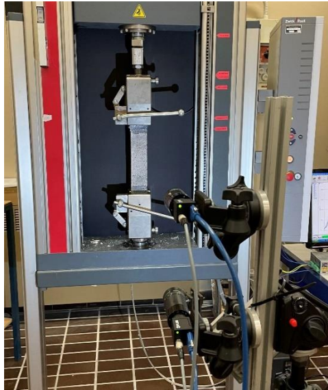
Figure 23. FRCM systems: tensile test setup.
