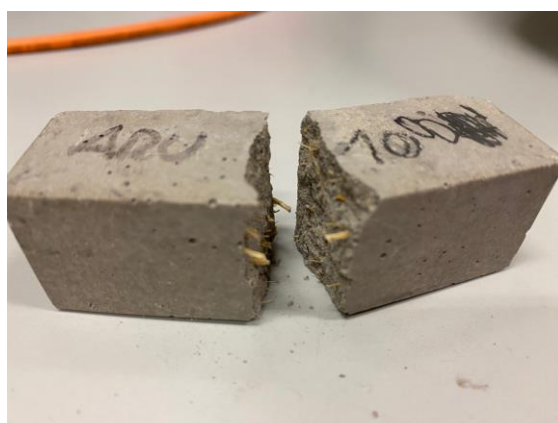
Figure 1. Image of a specimen of AAM reinforced with bamboo fibres after the flexural strength test
