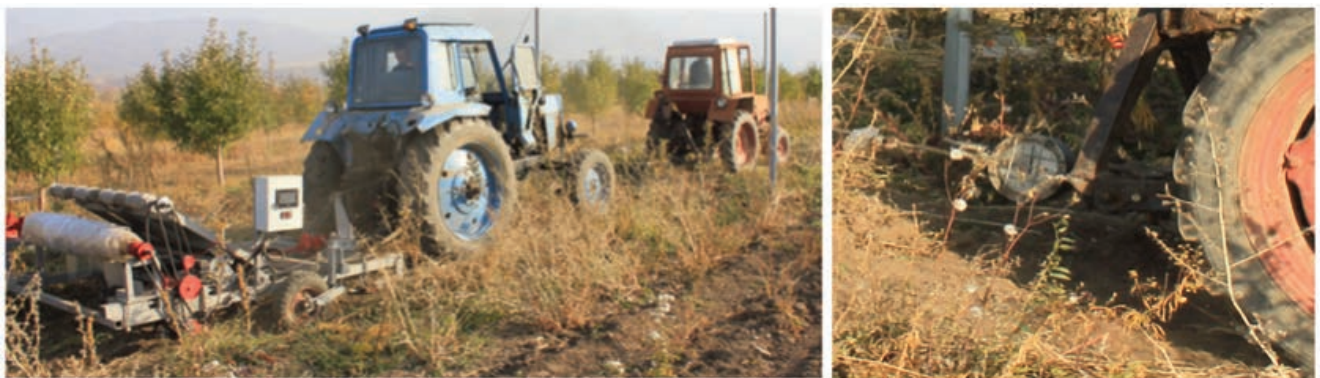
Figure 6. Measuring the traction resistance.
