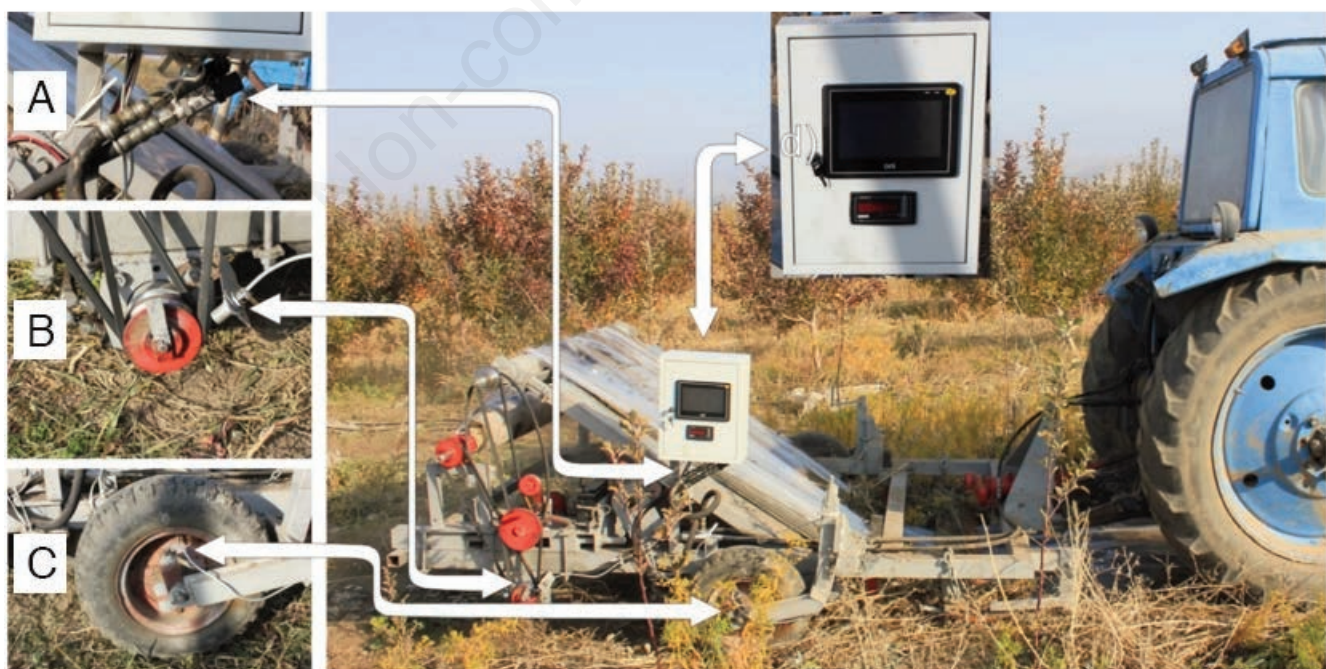
Figure 4. Sensors installed on the experimental unit: A) pressure sensor; B) sensor of the hydraulic motor speed; C) sensor of unit forward velocity; D) data logger with PC Interface.
