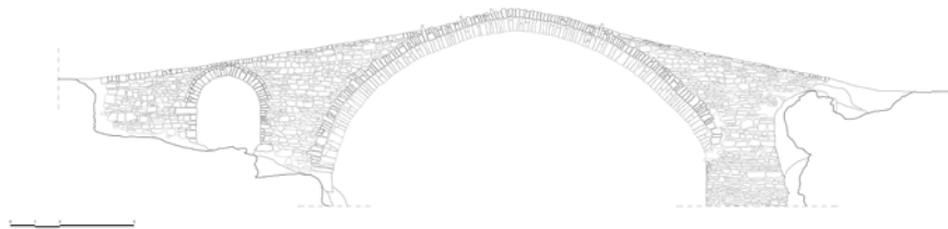
Figure I-5.1.2 The downstream facade of the Katiu Bridge.
