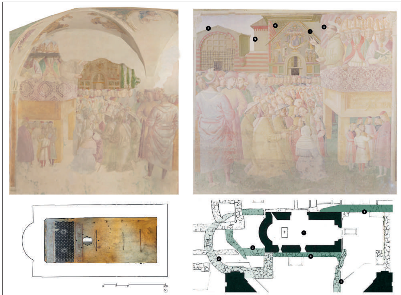
Fig. 6. Top left : Episode of the Proclamation of the indulgence at the Porziuncola , painted by Tiberio d'Assisi in the Chapel of the Roses in Montefalco. (Source: Authors). Bottom left : Plan of the vault of the Porziuncola obtained through integrated digital survey, showing the opening that allowed sound to reach people on the upper level. (Elaboration by the authors). Right : Archaeological stratigraphy around the Porziuncola (Source: Romanini 1989; Belardi, Menchetelli, Cotana 2024) compared with the buildings depicted in the fresco painted by Tiberio d'Assisi in the Chapel of the Roses at Santa Maria degli Angeli: 1. Porziuncola; 2. Choir of the lay people; 3. Choir of Saint Bernardino; 4. Wall of the convent; 5. Wall of the Sacrament Chapel; 6. Foundations of the portico. (Elaboration by the authors).
