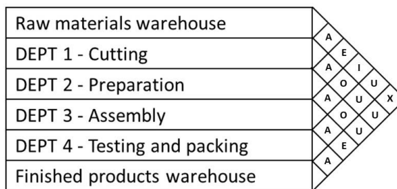
Figure 3: Buff diagram. The diagram shows the relevance of the proximity relationships between production departments (DEPTs) of the plant. The relevance levels are as follows: absolutely necessary (A), especially important (E), important (I), ordinary (O), unimportant (U), and undesirable (X).
