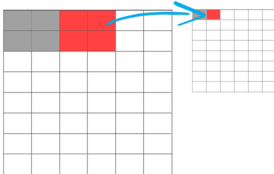
Figure 3: The size reduction process associates to a 2 \times 2 pixels area (on the left) a single pixel (on the right) having as value the mean value of the 2 \times 2 cell.
