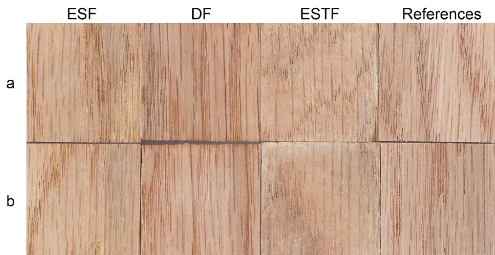
Figure 8. Oak samples after treatment with ESF, DF, or ESTF compared with the wood without coating as reference samples. (a) Virgin samples. (b) Samples pre-extracted in ethanol.
